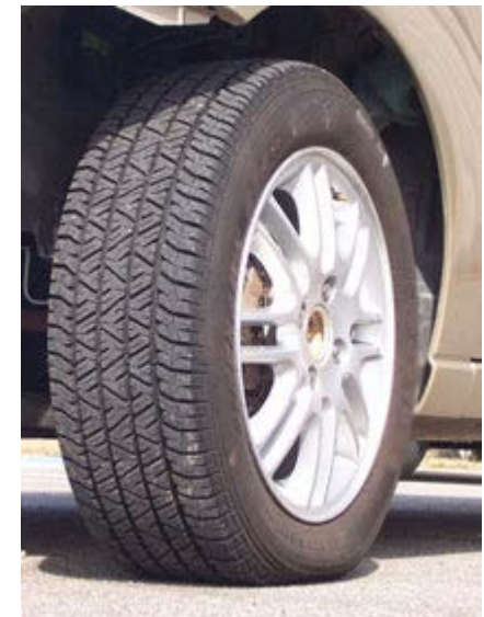
Tire at 16 psi 50% recommended pressure
