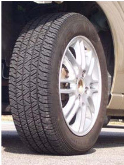
Tire at 32 psi 100% recommended pressure
